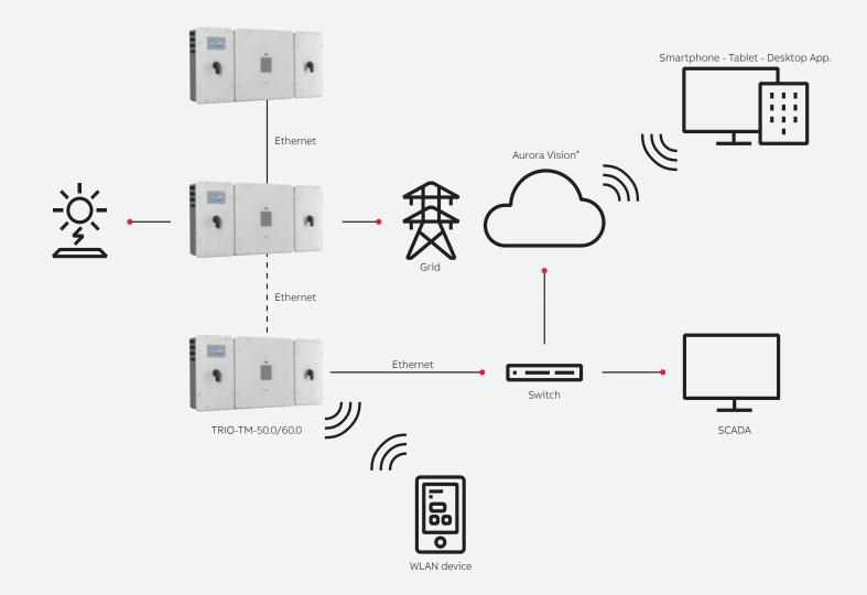
ABB TRIO-TM-50.0/60.0 string inverter block diagram
